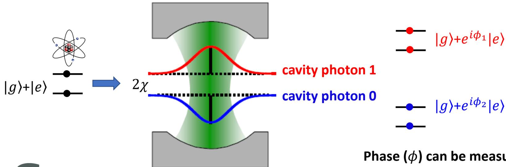
Phase ( $\phi$ ) can be measured by Ramsey interferometry.
