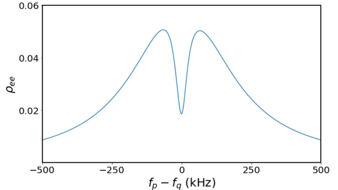
*Spectrum simulation of electromagnetically induced transparency. I used this simulation to fit the experimental data.*
