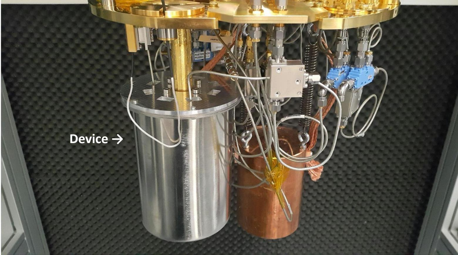
↳ To protect the device from radiation and magnetic noise.
