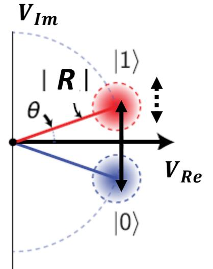
$$\text{reflection } (|R|) \sim \sqrt{V_{Re}^2 + V_{Im}^2}$$
