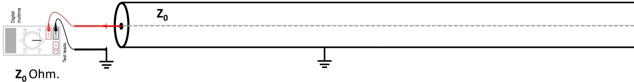
If you immediately readout the Ohm meter before the probe signal propagates...
