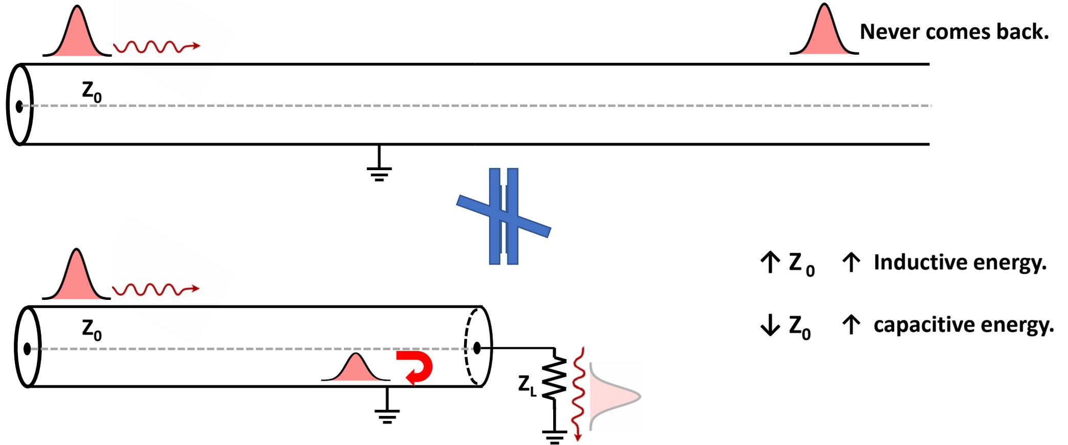
The pulse is totally dissipated when  $Z_0 = Z_L$  (Impedance matching).
