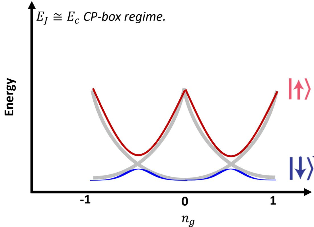
**half Integer  $n_g$**  Insensitive to charge noise (charge sweep spot).
