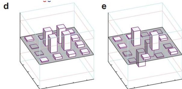
$$|\Phi^+\rangle = \frac{1}{\sqrt{2}} (|0, 1\rangle + |1, 0\rangle) \quad |\Phi^-\rangle = \frac{1}{\sqrt{2}} (|0, 1\rangle - |1, 0\rangle)$$
