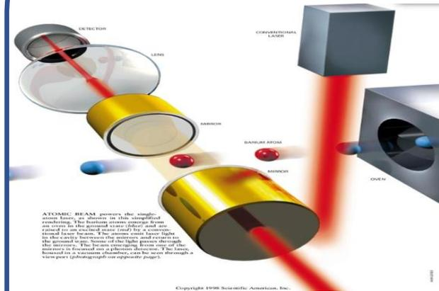
ATOMIC BEAM maser, the single-atom laser, is shown in this simplified rendering. The atomic stream originates from an oven on the right and is directed and controlled by a magnetic field. A microwave beam is directed through the atoms and is reflected by the mirror. The beam emerging from one of the detectors is directed to a detector. The image is a photograph of the maser. Copyright 1998 Scientific American, Inc.
